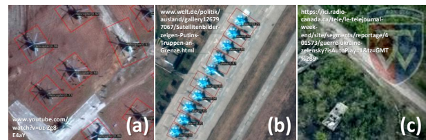
Figure 8: Qualitative analysis of an AMOD-trained detector on unseen real-world RGB imagery containing military equipment on real-world RGB satellite photographs released through public news coverage of the Russia–Ukraine war: (a) and (b): Successful detections of helicopters and airplanes. (c): A failure case of detecting tanks.
